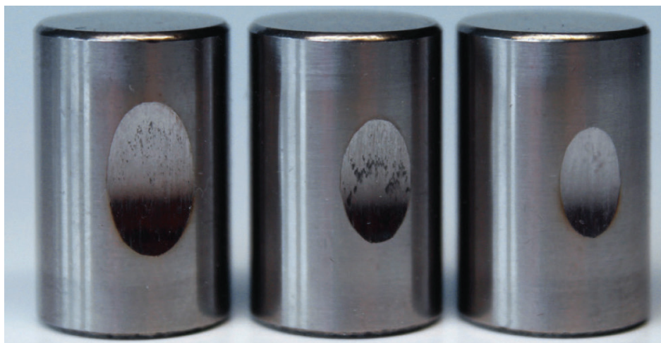
Figure 2: Test Cylinders After Reichert Wear Test
