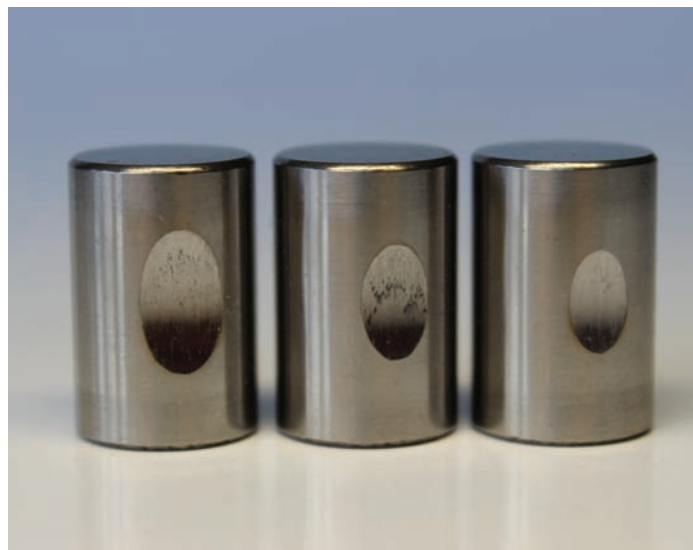
Test cylinders after Reichert Abrasive Wear Test using (left to right) water, 5 percent solution of a commercially available cooling lubricant, and 5 percent solution of Novotec CL800. (Photo: Gelita)
