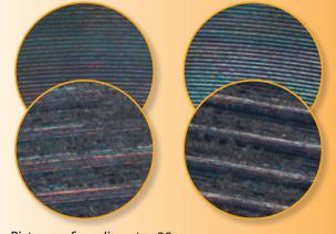
Piston surface diameter 60 mmConventional coolant with<br/>5% oil leaves residuesClean<br/>of
