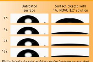
Wetting behavior of a water droplet on a steel surface (cross sectional view).
