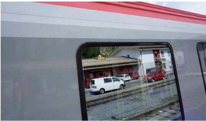
IMAGE 3 and 4: Sparkling windows and paintwork: the protective film on ÖBB train carriages makes the vehicle's exterior look "like new"
