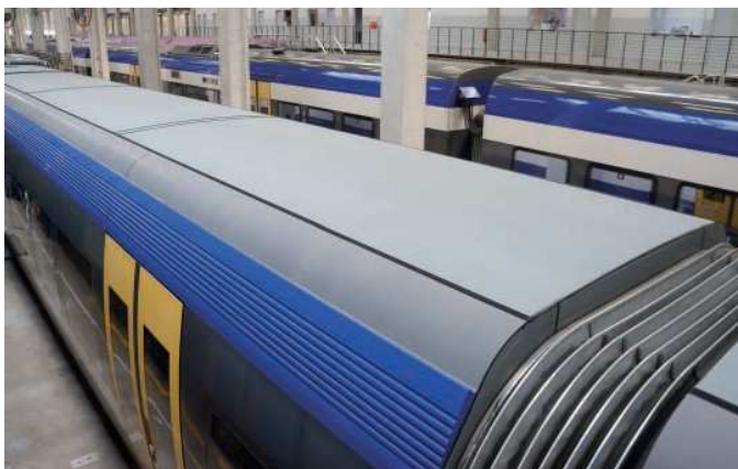
IMAGE 1: Clean as a result of self-cleaning: the roofs of NOB train carriages
