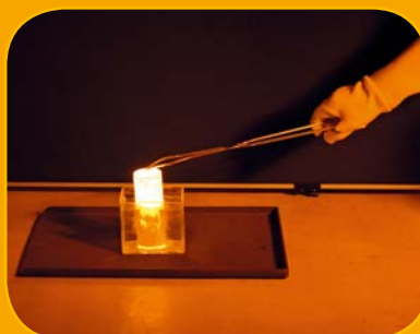
Thermal shock test of a 1200 °C hot burner nozzle in water.
